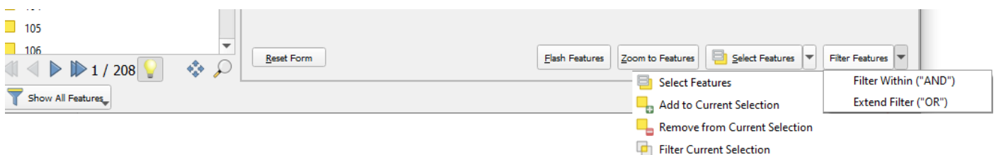
Pic. 87 Select/filter features using form in QGIS data attribute table – other options.
