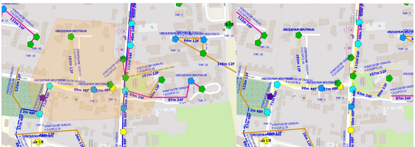
Pic. 60 Selecting features by polygon in QGIS. Selection polygon on the left and selected features on the right.
